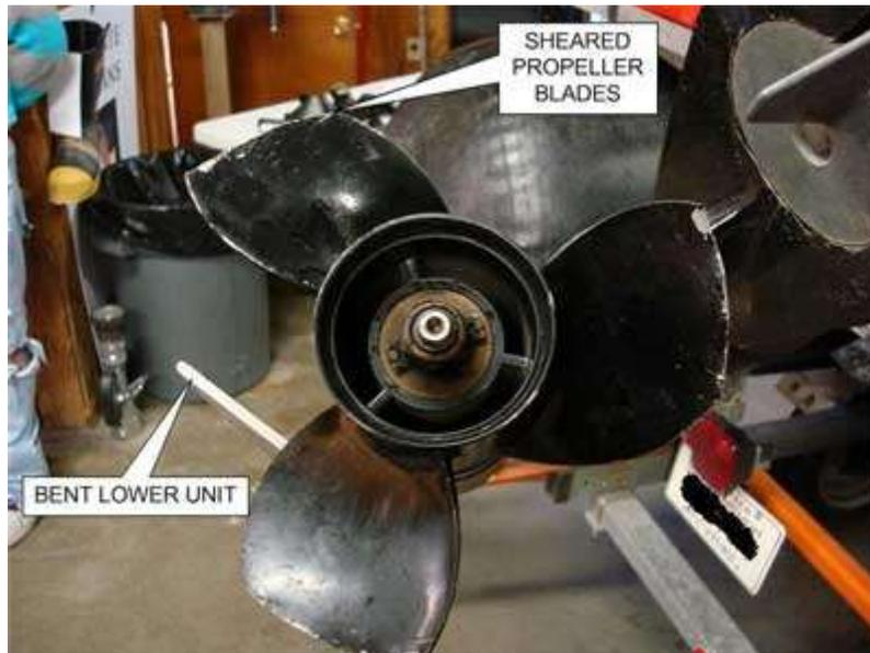
**Photo 1. Picture of damaged lower unit and propeller.
