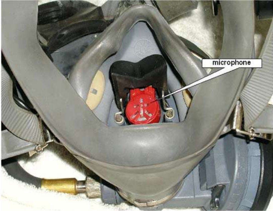
Photo 3. Example of microphone that was not working
