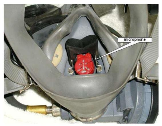
Photo 3. Example of microphone that was not working
