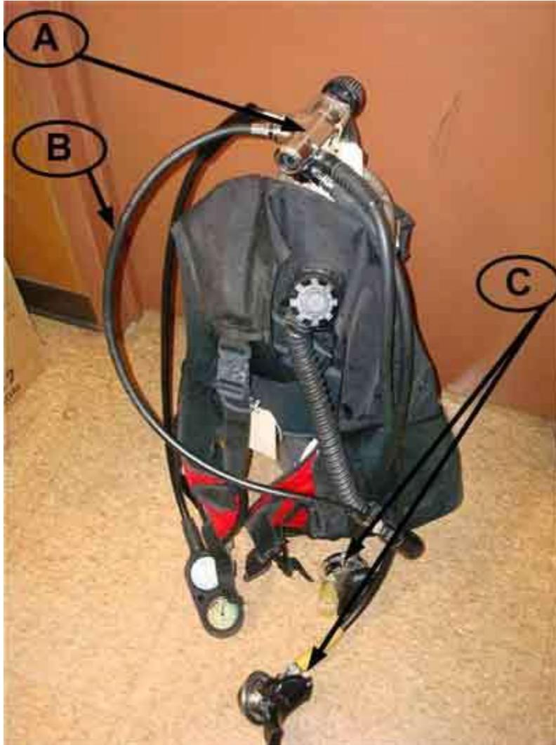
**Photo 1. Victim' s SCUBA gear. First-stage regulator (A) attached to tank valve upside down, resulting in the intermediate-pressure auto-fill hose (B) profiling across the victim' s chest instead of over the left shoulder. Primary second-stage and octopus regulator (C) incorrectly profiling off the left side of the victim resulting in the incorrect mouthpiece orientation (upside- down exhaust valve), possibly creating a breathing air complication underwater.**
