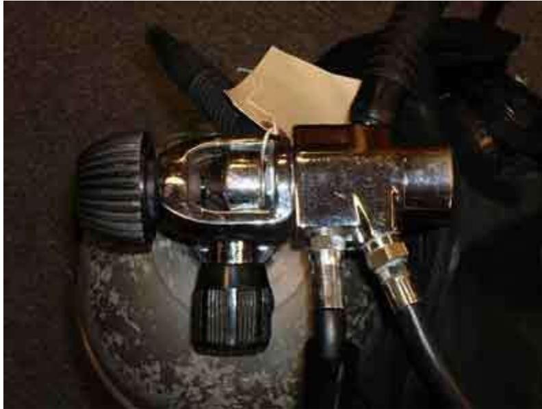
**Photo 2. First-stage regulator attached at the cylinder valve incorrectly. The regulator block to the right of the valve should have been rotated 180 degrees so the second-stage hoses appearing at the top of this picture would have profiled at the bottom or the diver' s right side.**
