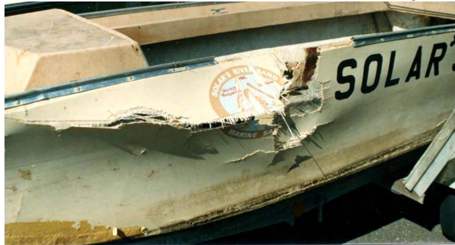
Figure 9-4 Photo of vaulted boat damage Source: Dr. William Chilcott
