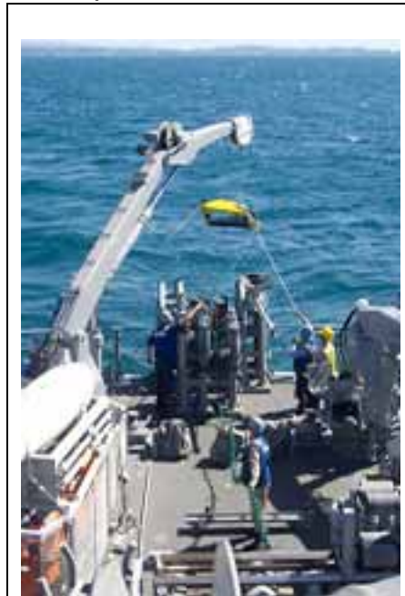
Klein System 5500 Side Scan Sonar Towfish being deployed from a US Navy MCM ship
