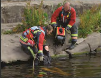
SARbot@ - rapid response rescue MiniROV system.
