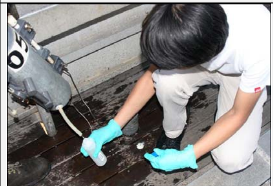
Water samples collected with Niskin bottle.
