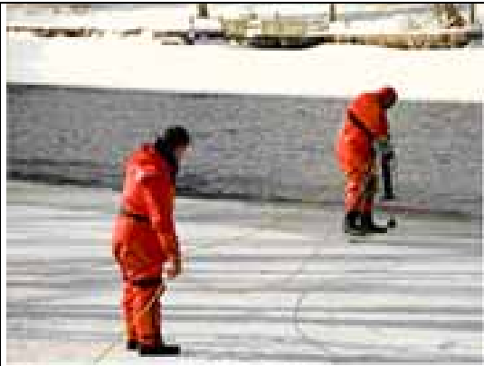
Team members work to move the sonar unit down river approx 50ft from the LSP to look for new targets. The Kongsberg Sonar Unit was suspended over the ice edge and secured with an ice screw
