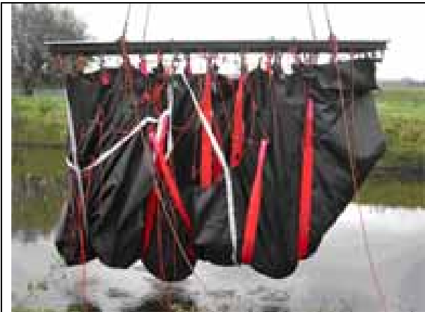
Recovery of a car that was too far gone to be lifted by crane the usual way. It was packaged underwater and then lifted.
